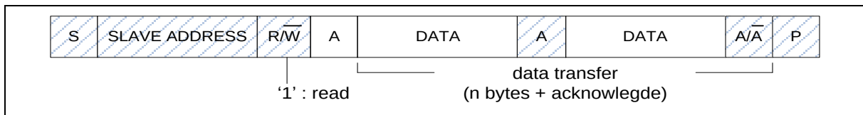
Figure 6.15-10 Master Reads Data from Slave with a 7-bit Address
